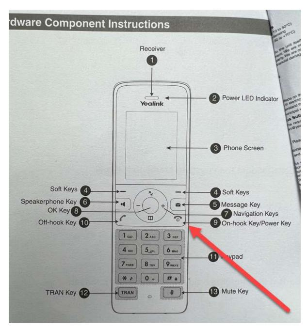
NB – the handset will NOT power off unless its removed from the charging cradle
